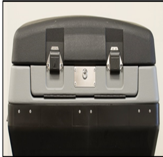
Figure 20 - Unhooked Latches on Scanning Unit
