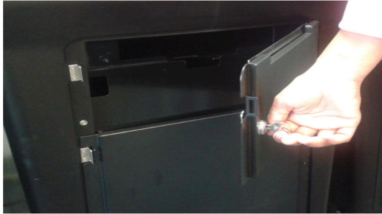
Figure 44 - Opening the Emergency Ballot Compartment Door
