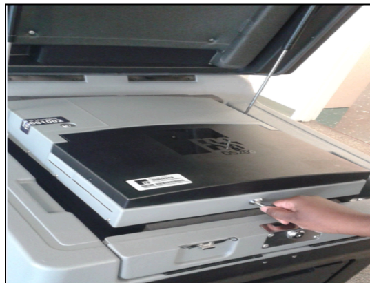
Figure 23 - Unlocking the Scanning Unit
