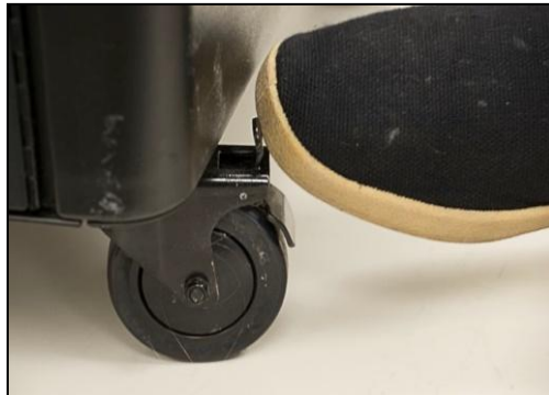
Figure 71 - Releasing the Brakes on the Scanning Unit
