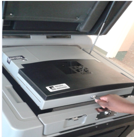
Figure 64 - Locking the Screen on the Scanning Unit
