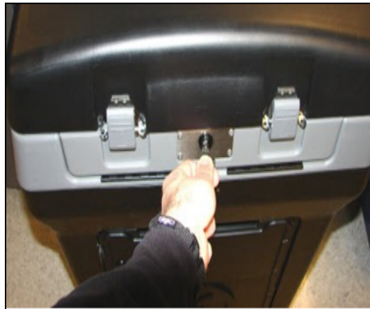
Figure 19 - Unlocking the Lid on the Scanning Unit
