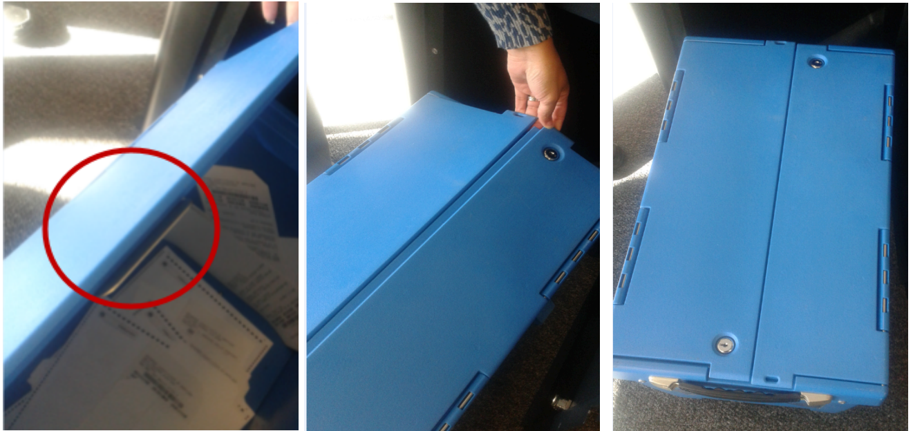
Figure 49 - "Tongue-in-groove" Fit on the Ballot Transfer Bin
