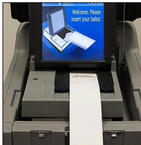
Figure 35 - Top Slot of the Scanning Unit and Ballot Activation Card
