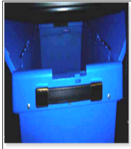
Figure 11 - Empty Ballot Transfer Bin in Main Ballot Box of the Scanning Unit
