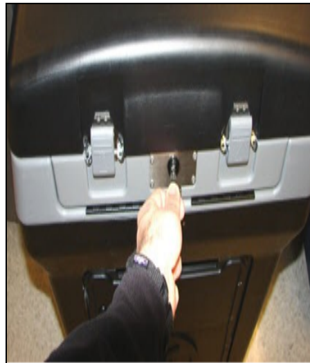
Figure 65 - Locking the Lid of the Scanning Unit
