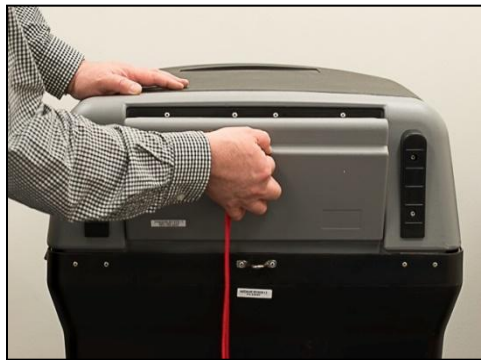
Figure 4 - Picture of Unlocking the Scanning Unit
